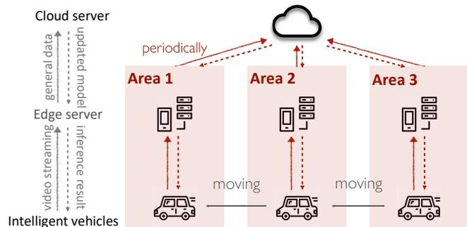
Fig. 1: The Edge Computing Framework for Intelligent Road Sensing Services
